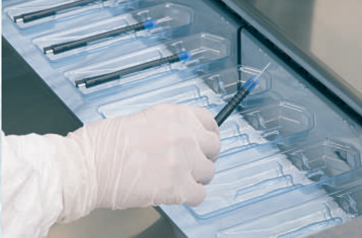
Cleanroom packaging of sterile single-use handpieces.
